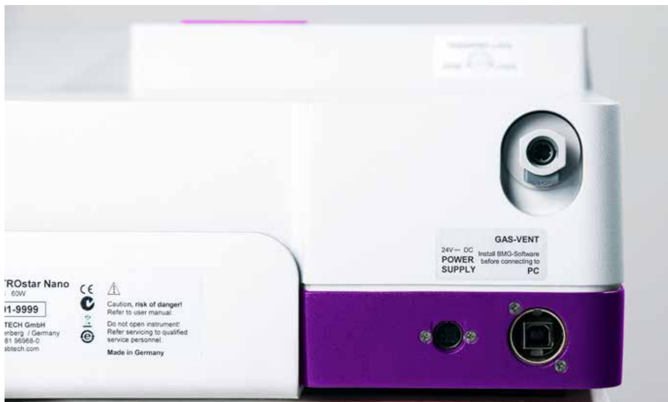
The gas vent can be used to purge the microplate chamber with a specific gas or gas mixtures.
